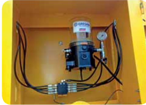
SENSÖRLÜ OTOMATİK YAĞLAMA SİSTEMİ AUTOMATIC LUBRICATION WITH SENSORS
