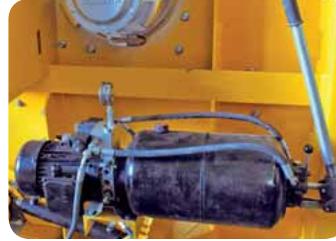
HİDROLİK ALT KAPAK SİSTEMİ VE MANUEL KAPAK AÇMA KOLU HYDRAULIC DISCHARGE GATE, AND MANUAL ARM FOR OPENING
