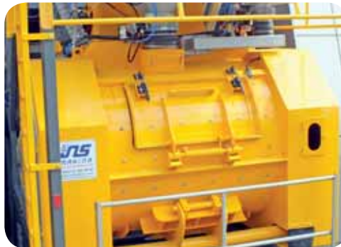
YAY BASKILI AMORTİSÖRLÜ GENİŞ SERVİS KAPAĞI SERVICE GATE WITH SPRING AND SHOCK ABSORBER.
