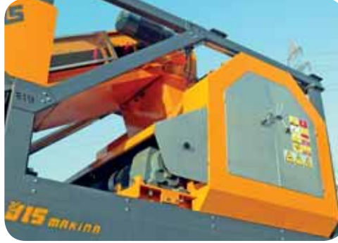
AÇILIR AGREGA GİRİŞ BOĞAZI OPENABLE AGGREGATE INLET.
