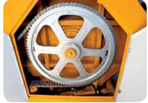
EN DAYANIKLI GÖVDE, ZİNCİR DİŞLİ, ZİNCİR VE PİNYON DİŞLİSİ HEAVY FRAME, CHAIN GEARWHEEL, PINION SHAFT, RINGS.
