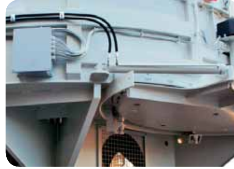
HİDROLİK ALT KAPAK SİSTEMİ HYDRAULIC BOTTOM GATE SYSTEM
